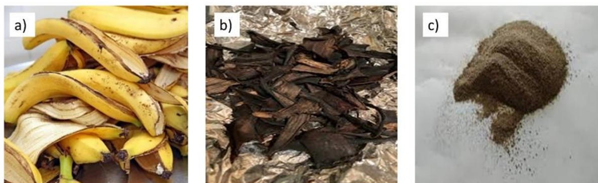
Figure 1. Preparation of banana peel powder: a) fresh banana peel, b) dried banana peel and c) dried banana peel powder.
