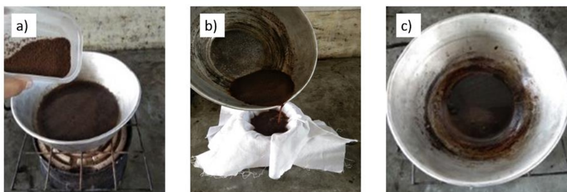
Figure 2. Preparation of banana peel paste: a) boiling the banana peel powder, b) filtering the liquid, and c) banana peel paste.
