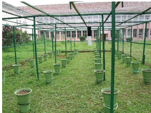
Plate 1: Experimental site with 44 pots before commencing experiment. Tiny Tag® air temperature and humidity data logger was hung 1.5 m above the ground level, in an open PVC cylinder which was painted with black and white paints (center of the image), in order to protect the probe from direct sun light.
