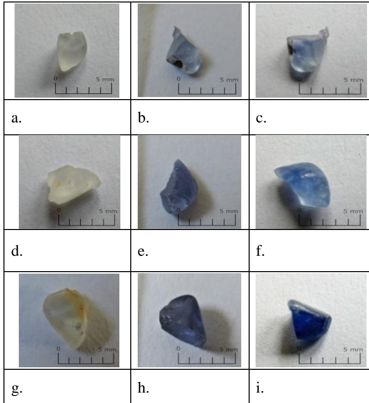
Figure 1: Colour changes of Geuda stones with different temperatures and soaking times. a. Unheated stone, b. Gas heat treatment ( 1750^{\circ}\text{C} ). c. Combined heat treatment (Electric Heat treatment after gas heat treatment) (3 Days of Soaking time and maximum temp of 1700^{\circ}\text{C} ) d. Unheated stone, e. Gas heat treatment ( 1750^{\circ}\text{C} ). f. Combined heat treatment (Electric Heat treatment after gas heat treatment) (1 Week of Soaking time and maximum temp of 1700^{\circ}\text{C} ). g. Unheated. h. Gas heat treatment ( 1750^{\circ}\text{C} ). i. Combined heat treatment (Electric Heat treatment after gas heat treatment) (1 month of Soaking time and maximum temp of 1700^{\circ}\text{C} )
