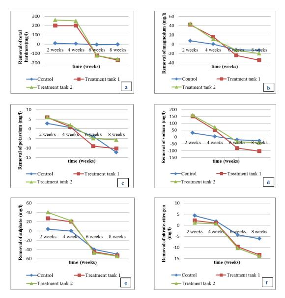
Figure 1: Changes in removal of components of water in the proposed treatment system containing floating aquatic plants with time; (a) Total hardness, (b) Magnesium, (c) Potassium, (d) Sodium, (e) Sulphate, (f) Nitrate-nitrogen
