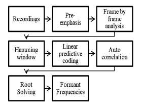
Scheme1 - Block diagram of the experiment setup of formant extraction
